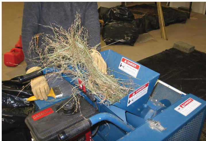
A farmer at the GNPC uses a thrasher to clean seed (switchgrass - panicum virgatum ) for the Founder Seed project.
