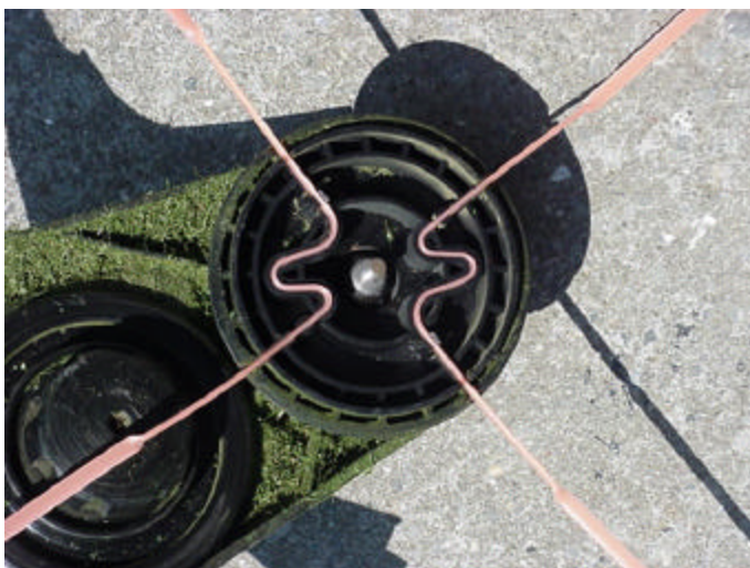
Underside of Aeroflex weed trimmer head and blade attachment.
