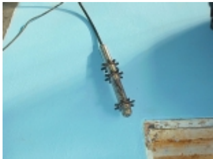
The head of the See Snake is equipped with a camera.
