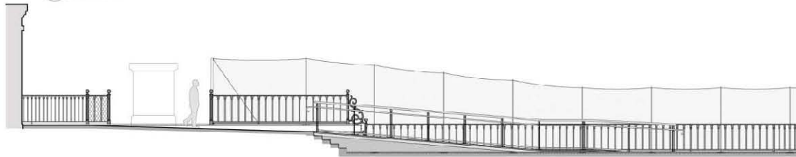
1 A-2 PARTIAL PLAN & ELEVATION OF FENCE & RAILING AT MANHATTAN SCALE: 1/8" = 1'-0"
